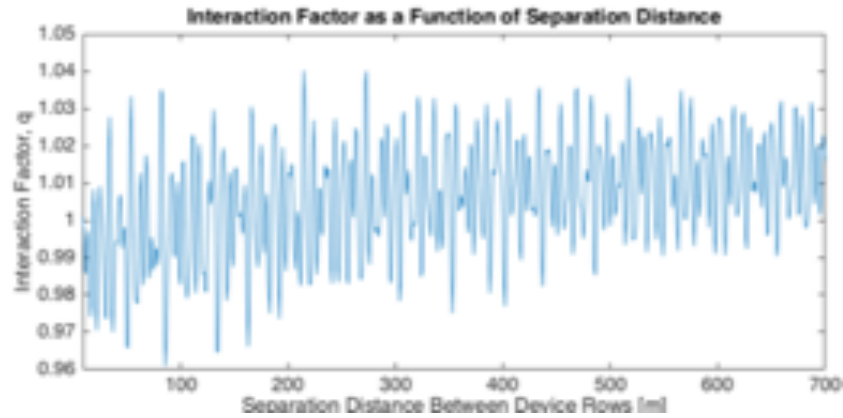
Figure 5.7: Interaction factor as a function of distance between offset rows for a 60x700 meter space
