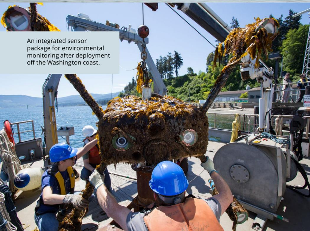
An integrated sensor package for environmental monitoring after deployment off the Washington coast.
