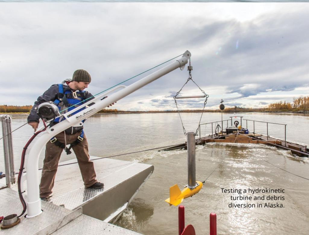
Testing a hydrokinetic turbine and debris diversion in Alaska.
