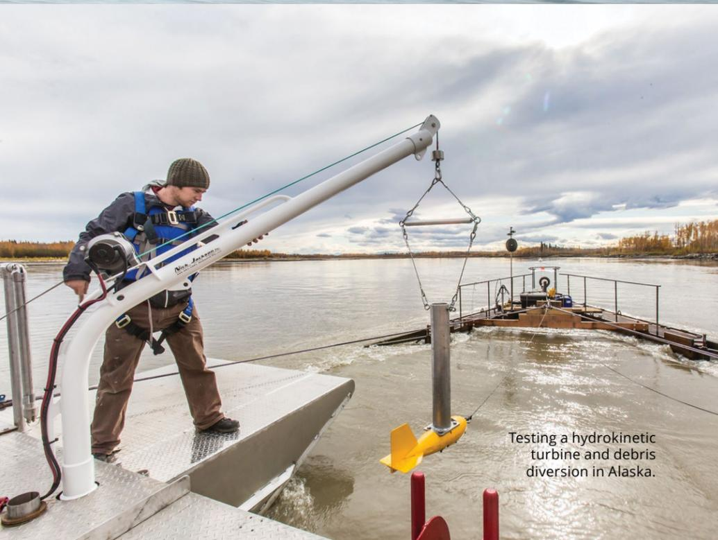
Testing a hydrokinetic turbine and debris diversion in Alaska.
